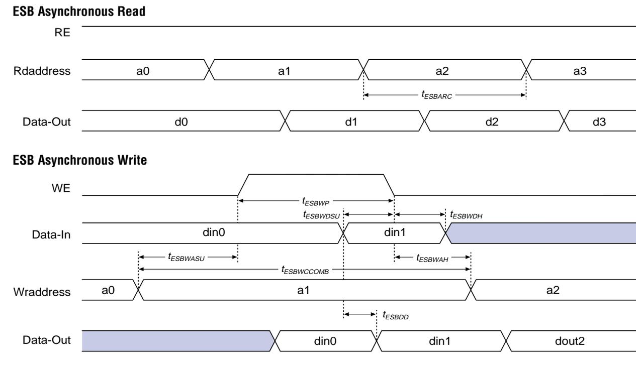
Figure 39. ESB Synchronous Timing Waveforms
