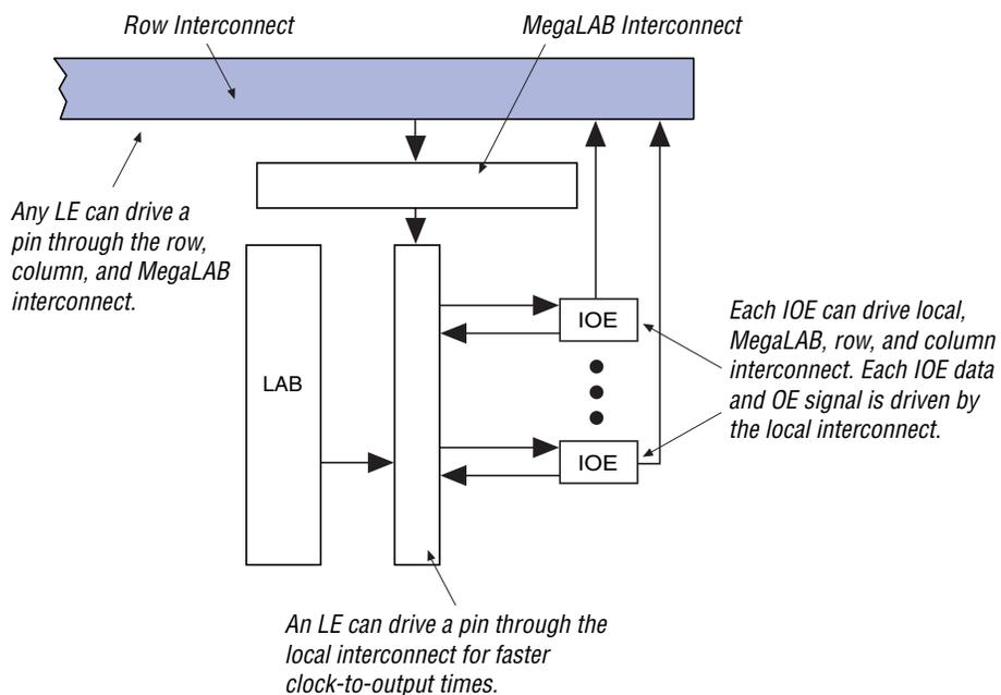
Figure 28 shows how a column IOE connects to the interconnect.
