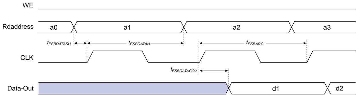
**ESB Synchronous Write (ESB Output Registers Used)**
