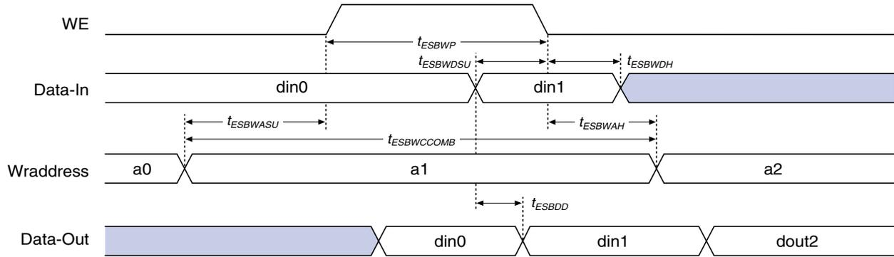
Figure 34. ESB Synchronous Timing Waveforms
