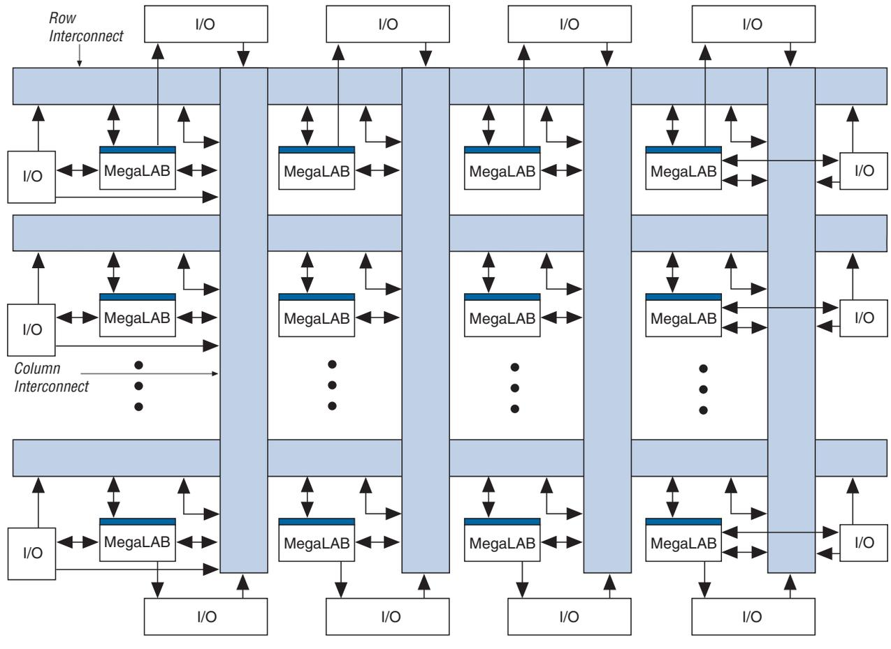
A row line can be driven directly by LEs, IOEs, or ESBs in that row. Further, a column line can drive a row line, allowing an LE, IOE, or ESB to drive elements in a different row via the column and row interconnect. The row interconnect drives the MegaLAB interconnect to drive LEs, IOEs, or ESBs in a particular MegaLAB structure.
