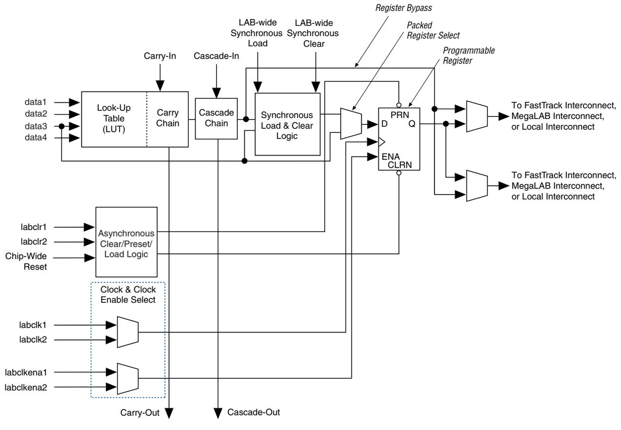
Each LE's programmable register can be configured for D, T, JK, or SR operation. The register's clock and clear control signals can be driven by global signals, general-purpose I/O pins, or any internal logic. For combinatorial functions, the register is bypassed and the output of the LUT drives the outputs of the LE.
