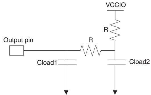
**Figure 38. AC Test Conditions for the LVDS I/O Standard**
