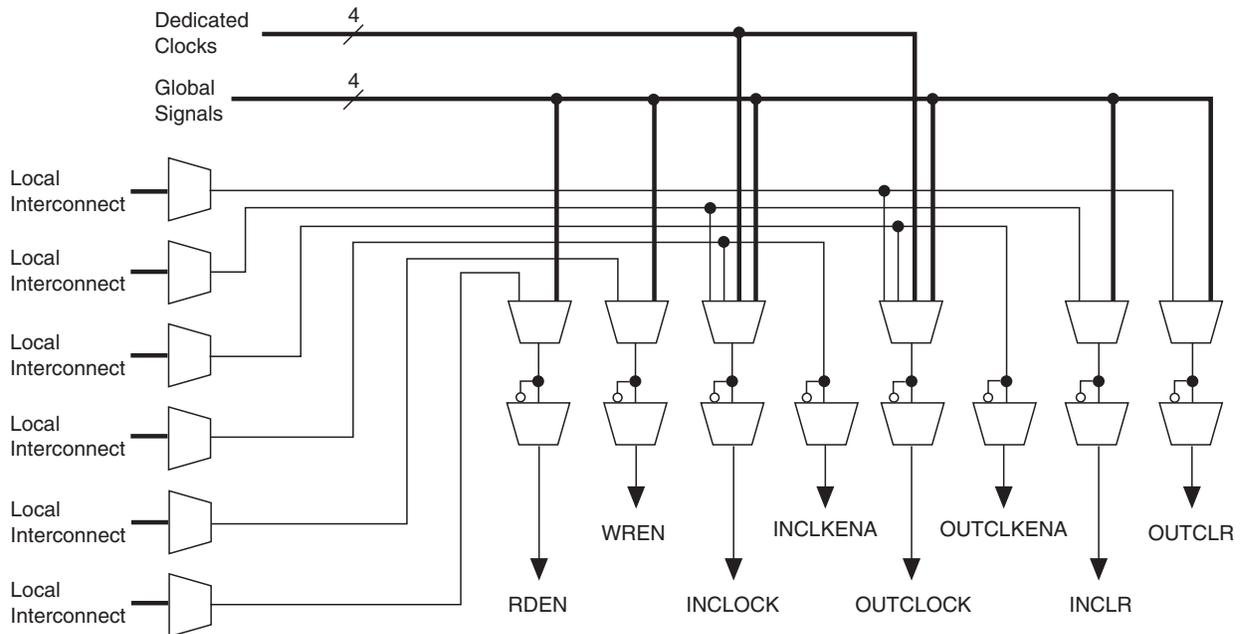
An ESB is fed by the local interconnect, which is driven by adjacent LEs (for high-speed connection to the ESB) or the MegaLAB interconnect. The ESB can drive the local, MegaLAB, or FastTrack interconnect routing structure to drive LEs and IOEs in the same MegaLAB structure or anywhere in the device.
