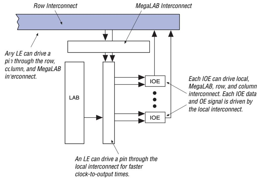
Figure 27 shows how a column IOE connects to the interconnect.
