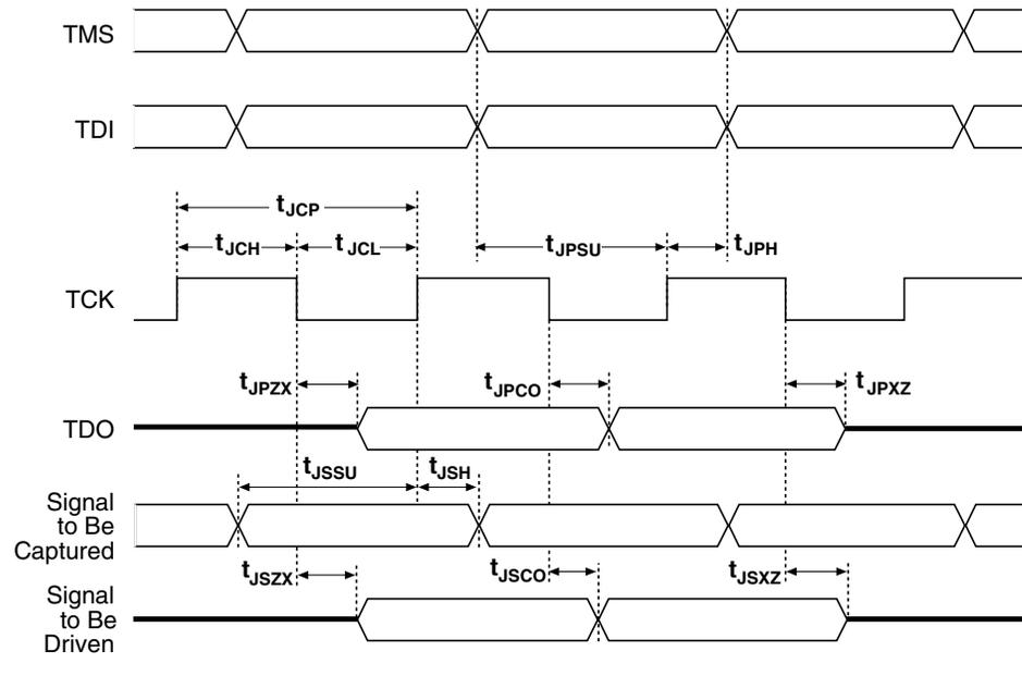
Table 16 shows the JTAG timing parameters and values for APEX 20KC devices.
