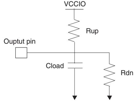
**Figure 37. AC Test Conditions for SSTL-3 Class I & II I/O Standards**
