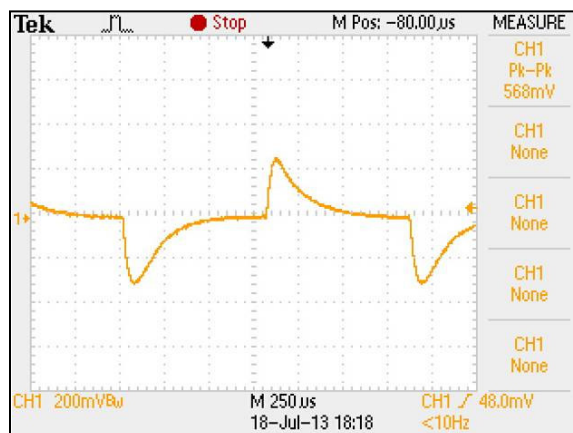
Figure 31: ERM02H72 Transient Response Vin = 72Vdc Load: Io = 100% to 75% load change Ch 1: Vo
