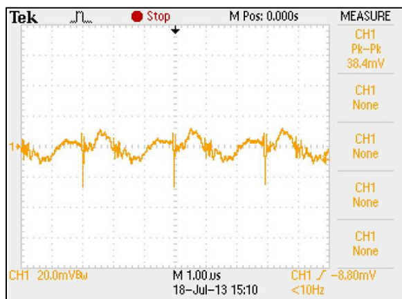
Figure 12: ERM04B72 Typical Output Ripple and Noise. Vin = 72Vdc Load: Io = 4.17A Ch 1: Vo
