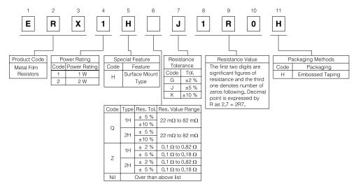
The above example shows a surface mount type metal film resistor, 1 W power rating, resistance value of 1.0 ohms, tolerance  $\pm 5$  %, and embossed taping.
