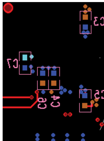
Figure 55. Bottom Layer decoupling
