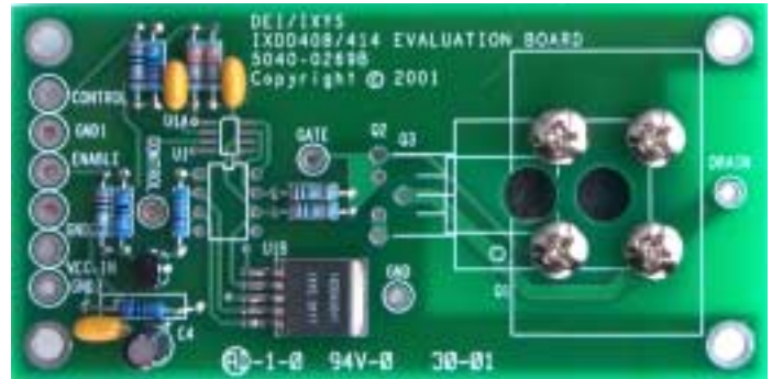
Figure 1 - EVDD408/EVDD409/EVDI409/EVDN409/EVDD414 Evaluation Board SOT-227 Device Installed For Illustration Purposes Only
