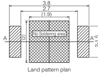
\* Soldering failure may occur depending on applied solder amount, so, please consider to use our recommended stencil and land pattern desing.
