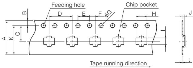
Taping condition : Lack of products in the middle of taping should be one MAX, but total quantity specified in the specifications should be secured.
