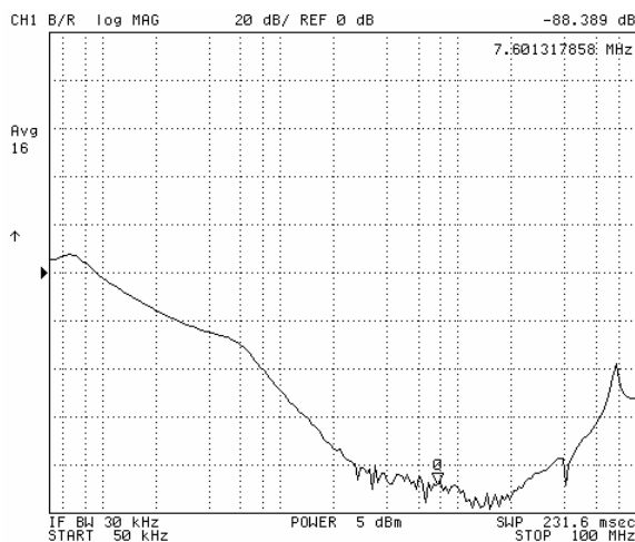
Fig. 3: Common Mode attenuation, 0.05-100MHz. Source and load resistances are 50Ω. Two 0.1μF Y-caps to common line. Vertical scale: 20dB/div, with zero dB level marked by arrow.
