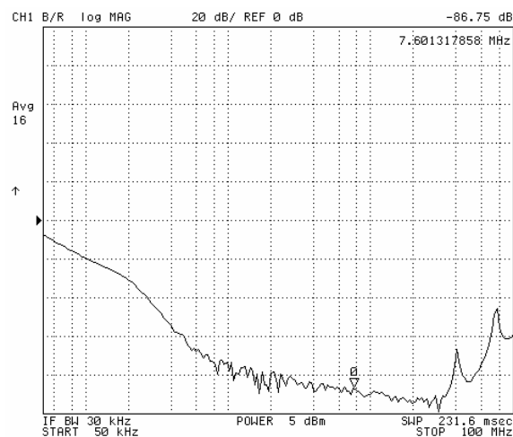
Fig. 4: Common Mode attenuation, 0.05-100MHz. Source and load resistances are 50Ω. Two 0.47μF Y-caps to common line. Vertical scale: 20dB/div, with zero dB level marked by arrow.
