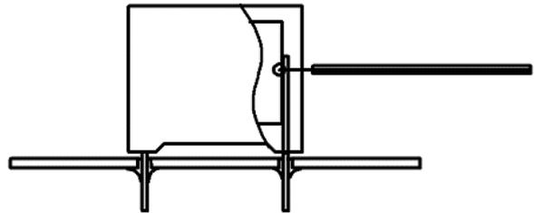
*Temperature monitored inside the capacitor.*
