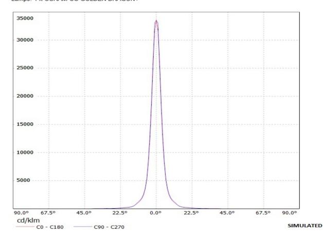
Luminaire: Ledil Oy FA10753\_LO2-D FA10753\_LO2-D Lamps: 1 x OSRAM-OS GOLDEN DRAGON+
