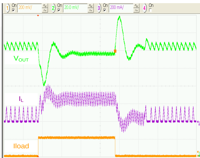
Figure 14. Load Transient 50 to 250mA, 3.6VIN, 5µs/div.
