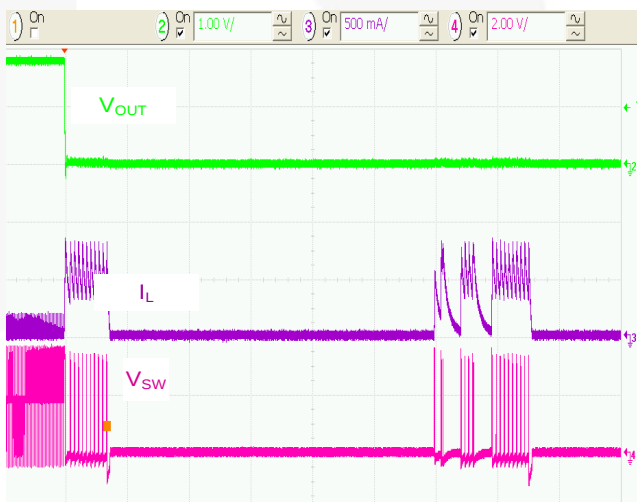
Figure 16. Metallic Short Applied at VOUT, 50µs/div.
