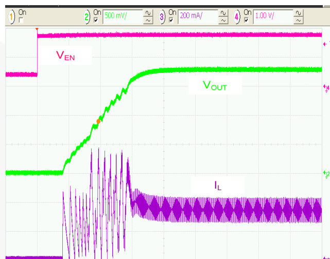
Figure 18. Soft-Start, R_{LOAD} = 6\Omega , 20µs/div.
