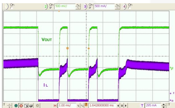
Figure 30. Over-Current, Load Increasing Past Current Limit, FAN53611
