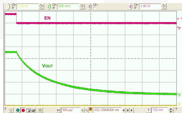
Figure 27. Shutdown, No Load, Output Discharge Enabled
