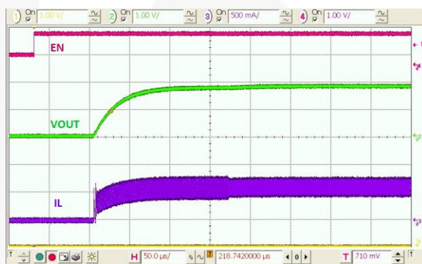
Figure 25. Startup, 3 \Omega Load
