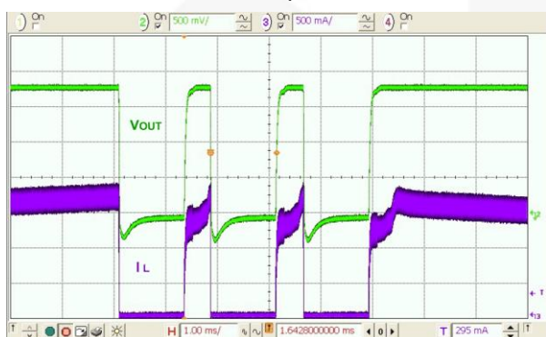
Figure 30. Over-Current, Load Increasing Past Current Limit, FAN53611
