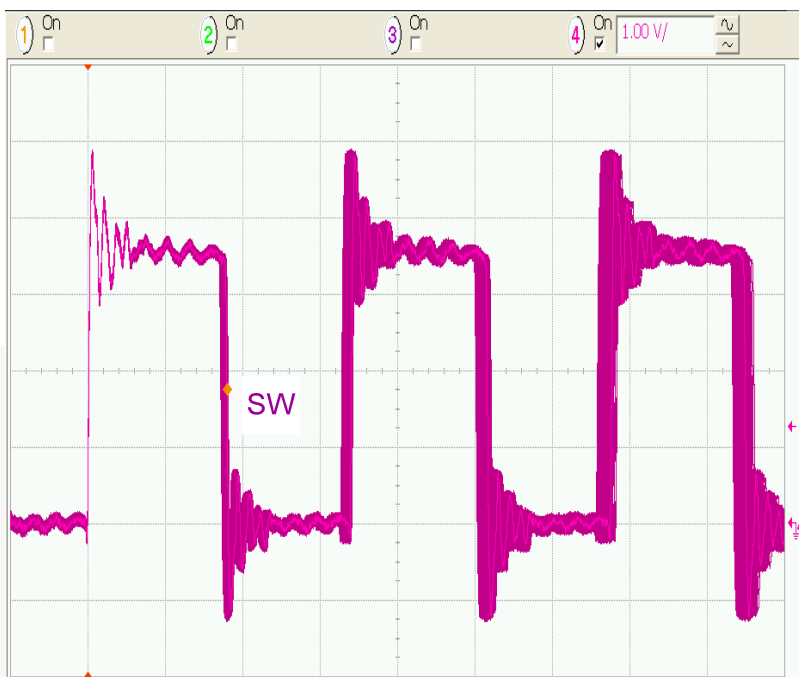
Figure 39. SW-Node Jitter (Infinite Persistence), I_{LOAD} = 200mA , 50ns/div.
