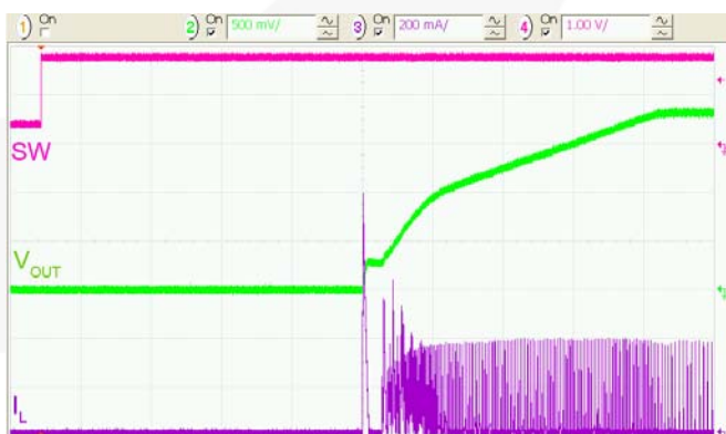
Figure 38. Soft-Start, R_{LOAD} = 50\Omega , 20\mu s/div.
