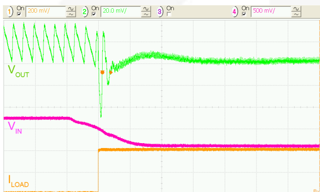
Figure 22. Combined Line/Load Transient 3.9 to 3.3\text{ V}_{IN} Combined with 40\text{ mA} to 400\text{ mA} Load Transient
