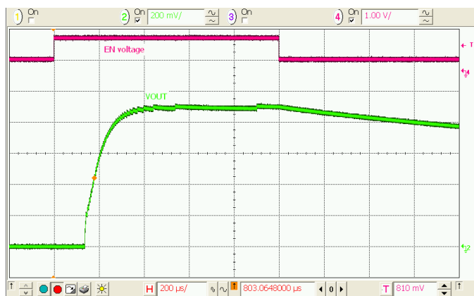
Figure 30. Startup / Shutdown, No Load, V_{OUT}=0.9\text{ V}
