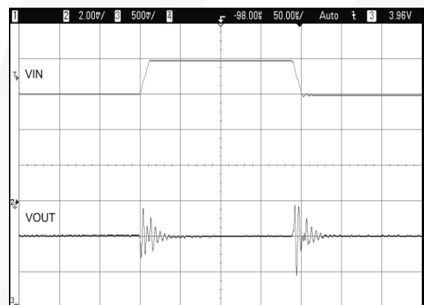
Figure 18. Line Transient V_{IN} = 3.7\text{ V} to 4.2\text{ V} , V_{OUT} = 1.0\text{ V} , 10\text{ }\Omega Load, 50\text{ }\mu\text{s/div} .
