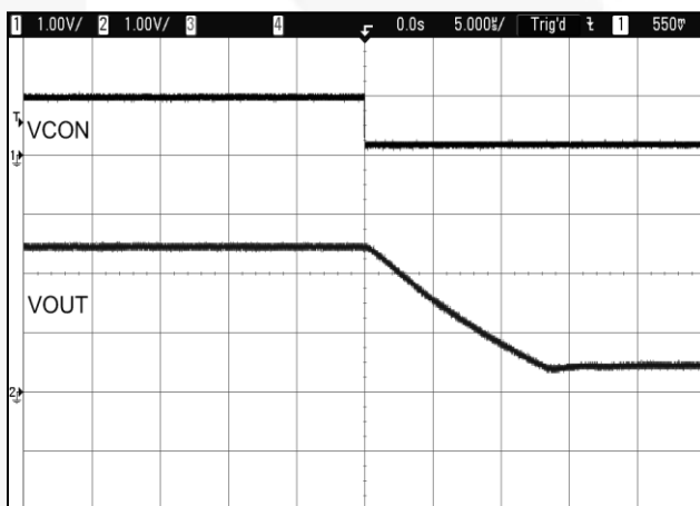
Figure 37. V_{OUT} Falling Transition 2.5 V to 0.5 V, V_{IN} = 3.7\text{ V} in Low-Power Mode
