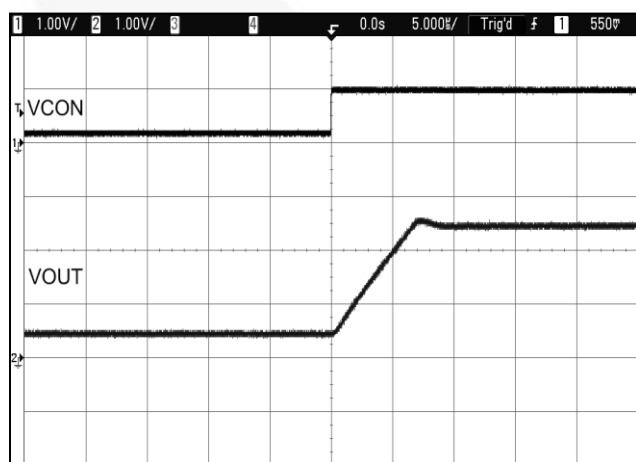
Figure 38. V_{OUT} Rising Transition 0.5 V to 3.0 V, V_{IN} = 3.7\text{ V} in High-Power Mode
