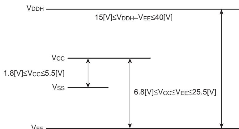
The recommended operating voltages are combinations within the shaded area in the figure below.
