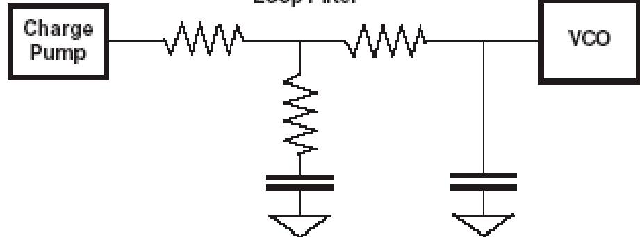
In PLL circuit applications, FCP SMT film capacitor advantages are tight tolerance on the capacitance value, stable capacitance with temperature, faster lock-up times, and no noise due to piezoelectric effects.
