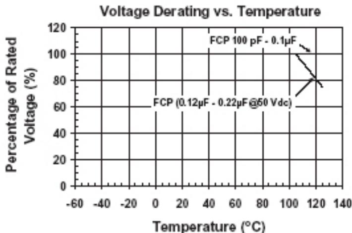
If the temperature on the surface of the capacitor is above 105°C, then the maximum voltage for FCP 50 Vdc ratings from .12  $\mu$ F to .22  $\mu$ F must be derated linearly from full rated voltage at 105°C to 75% of the rated voltage at 125°C.
