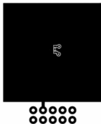
a. 60^\circ\text{C/W} when mounted on a 1 in 2 pad of 2 oz copper.
