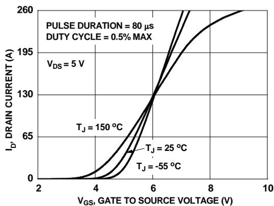
Figure 5. Transfer Characteristics
