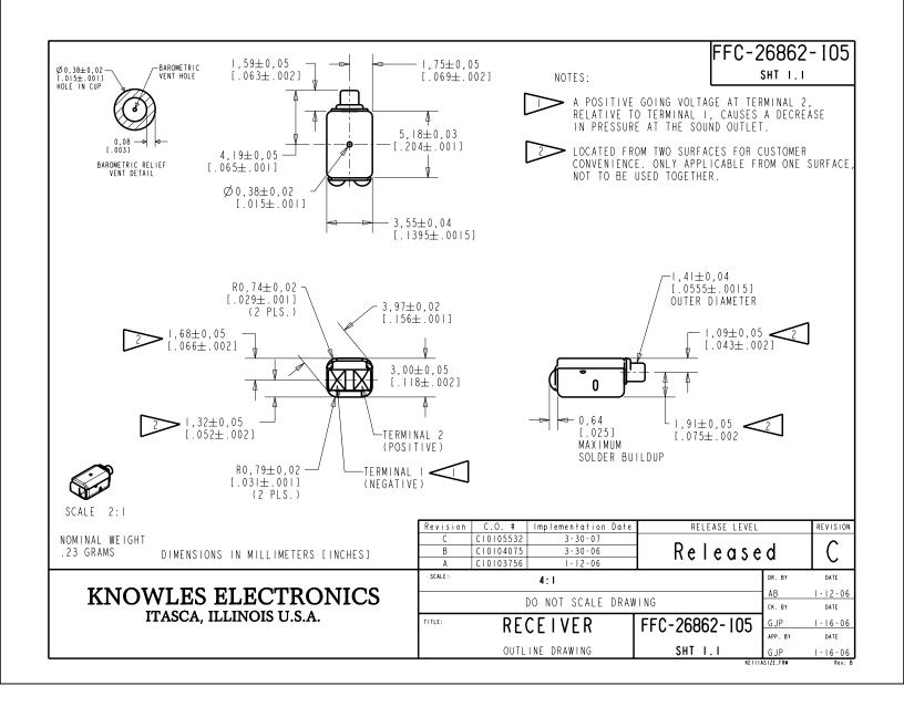
FERROFLUID AND TYPE III DAMPING FFC-26862-105
