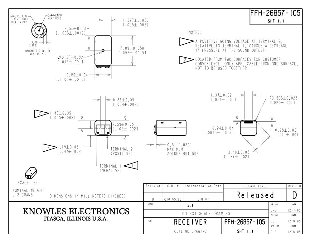
THE FFH-26857-105 IS A FERROFLUID DAMPED AND EXTERNALLY VENTED FH-6553 RECEIVER WITH A PEAK OF 5dB RELATIVE TO THE SENSITIVITY AT IKHZ UNDER CONSTANT VOLTAGE DRIVE CONDITIONS.
