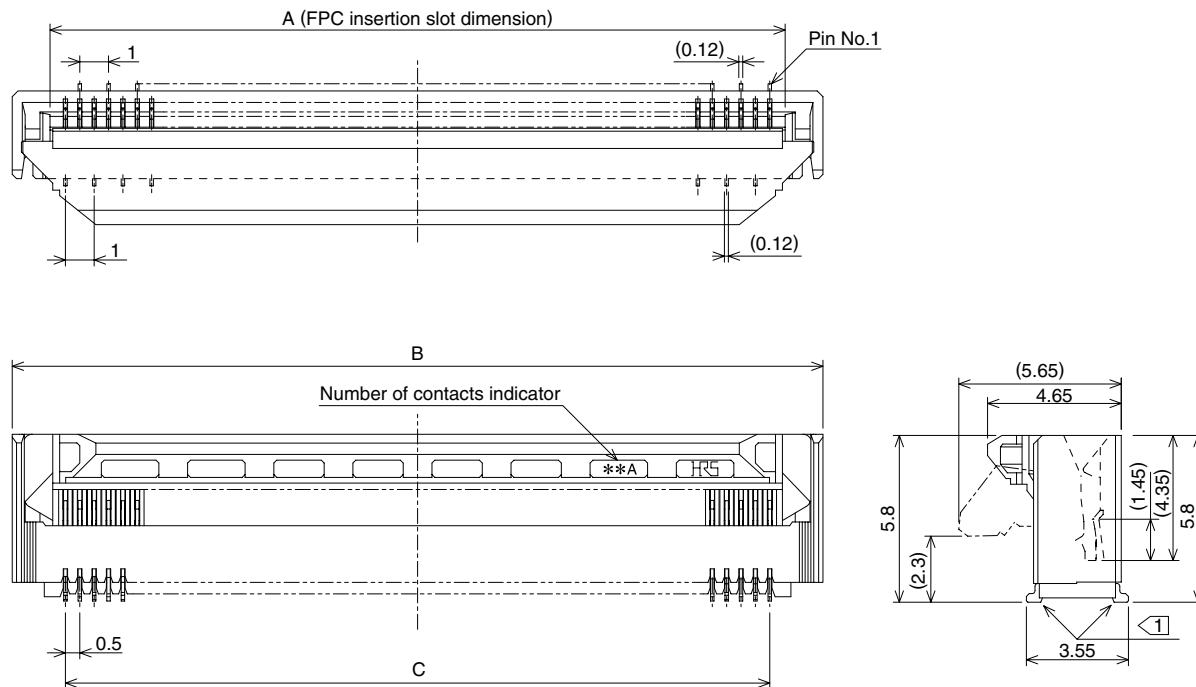
Note 1 : The coplanarity of each terminal lead within specified dimension is 0.1 mm Max.
