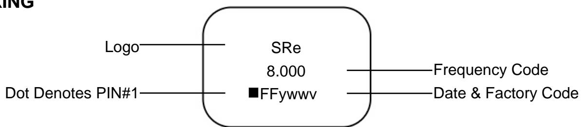
Below the marking diagram, five horizontal lines represent code components:
