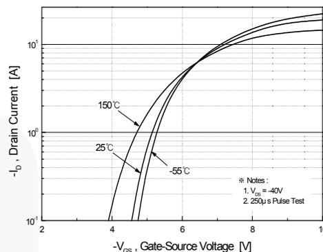
**Figure 2. Transfer Characteristics**
