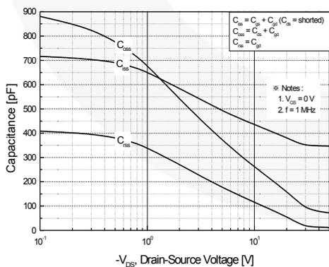
**Figure 5. Capacitance Characteristics**
