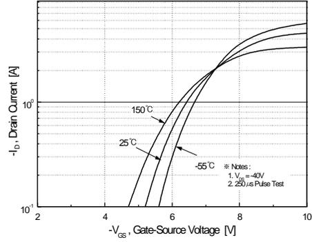
Figure 2. Transfer Characteristics
