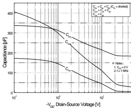
Figure 5. Capacitance Characteristics
