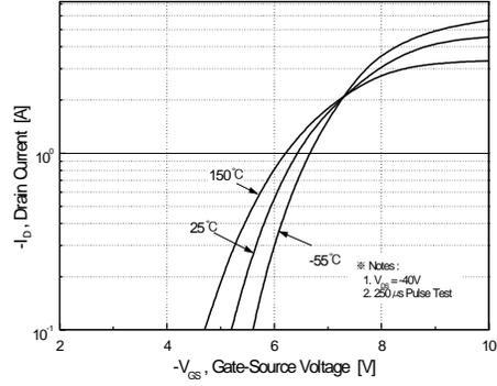
Figure 2. Transfer Characteristics
