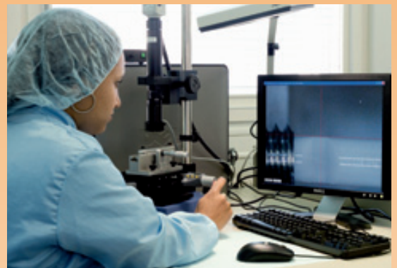
Clean room, inspection of fibre optic assembly
