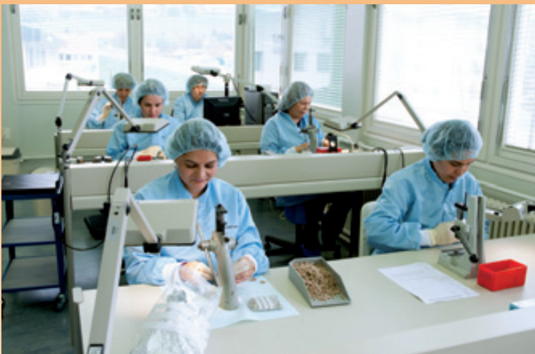
Clean room, assembly of fibre optic contacts
