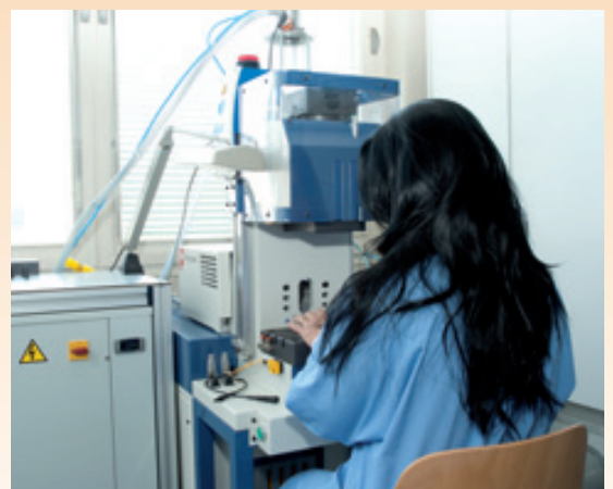
Over-moulding on cable
