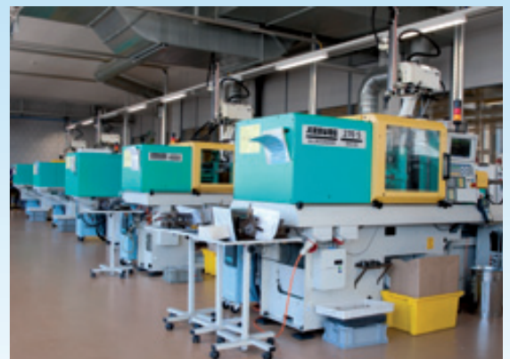
Injection of insulators
