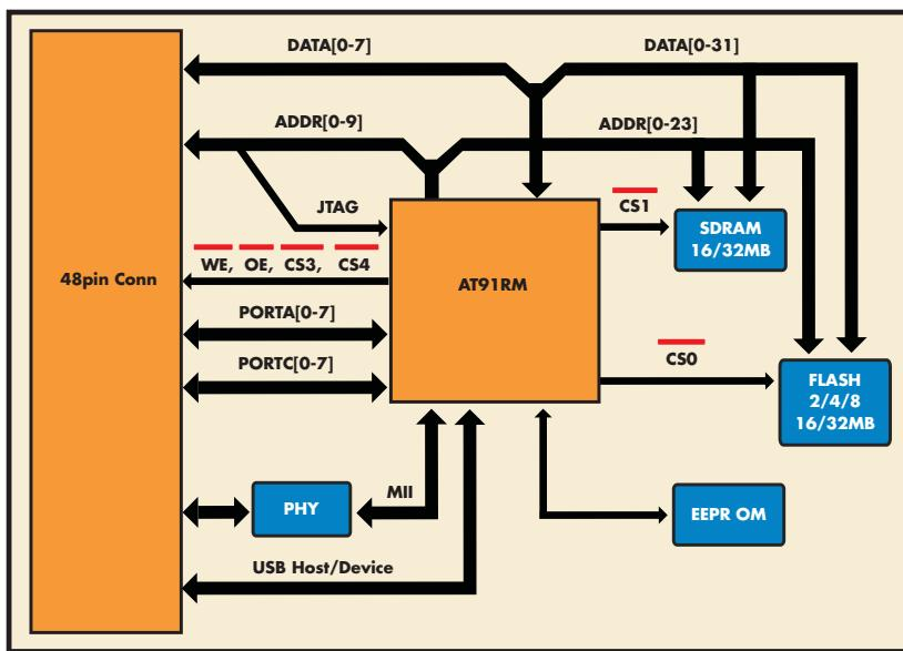
Universal 32-bit embedded core processor module offers a wide range of component connectivity options and pin-compatible upgrade options for designs using the ConnectCore™ 7U.
