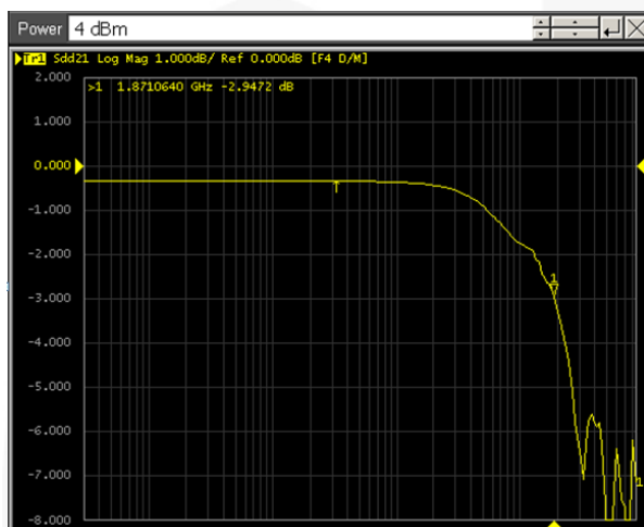
Figure 17. MHL Path SDD21 Insertion Loss Curve
