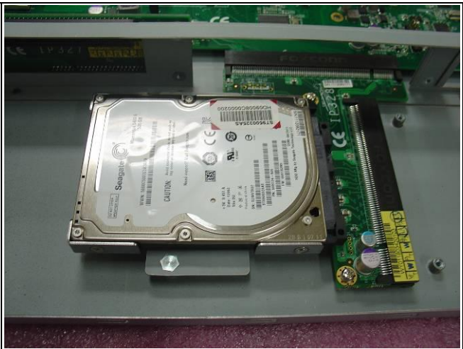
Fig. 9-4 Completion of HDD connection
