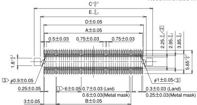
Note 1 Cross-hatched portions, totaling n places, indicate the ground circuits.
