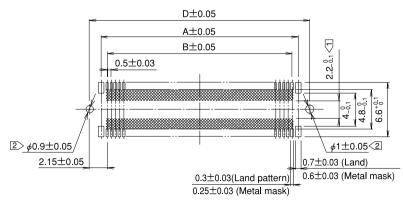
Note 1 The cross-hatched area inside the SMT land may come into contact with the connector contacts and thus care should be taken that the pattern does not extend beyond the SMT land width.
