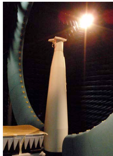
Free space antenna setup and Satimo SG64 3D-chamber.
