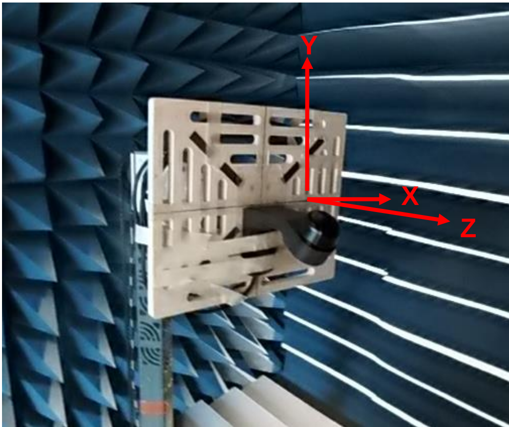
Figure.6 Testing Setup in ETS Anechoic Chamber
