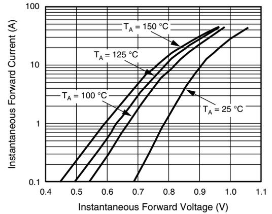
Figure 5. Typical Instantaneous Forward Characteristics Per Diode
