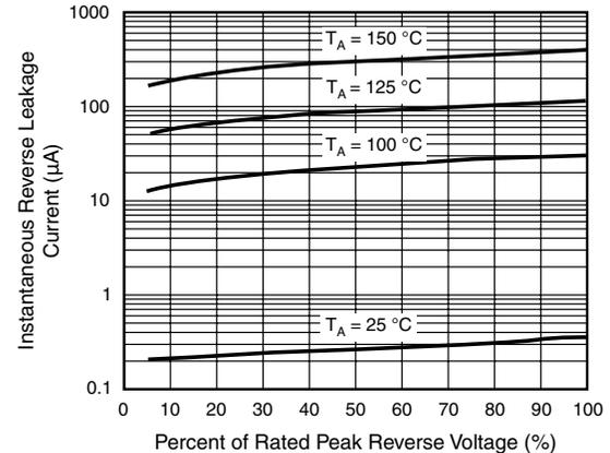
Figure 6. Typical Reverse Leakage Characteristics Per Diode
