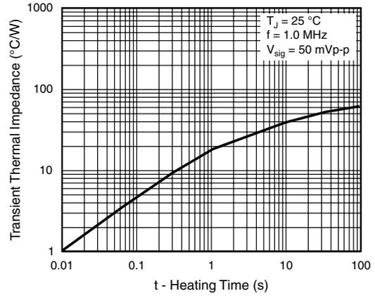
Figure 8. Typical Transient Thermal Impedance Per Diode
