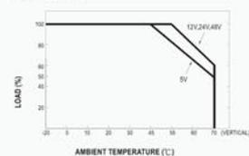
■ Output Derating VS Input Voltage
