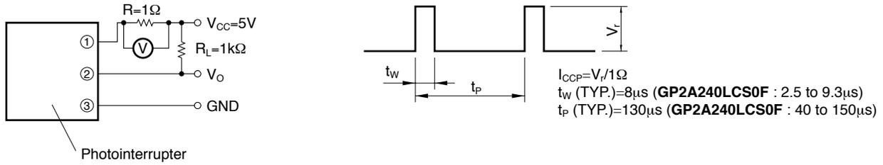
**Fig.2 Test Condition for Detecting Distance Characteristics**
