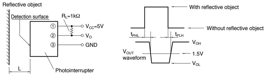
**Fig.4 Test Condition for External Disturbing Light Illuminance**
