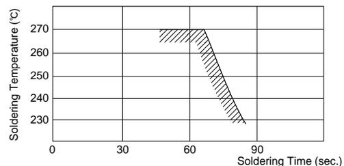
In case of repeated soldering, the accumulated soldering time must be within the range shown above.
