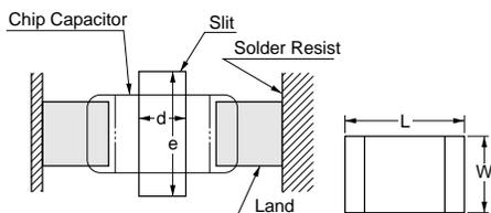
Preparing slit helps flux cleaning and resin coating on the back of the capacitor. But, the length of slit design should be shorter enough as much as possible to prevent the mechanical damage in the capacitor. The longer slit design might receive more severe mechanical stress from the PCB. Recommendable slit design is shown in the Table.
