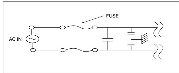
**4. Test Condition for AC Withstanding Voltage**
