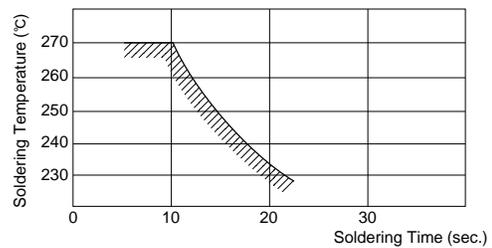
In case of repeated soldering, the accumulated soldering time must be within the range shown above.
