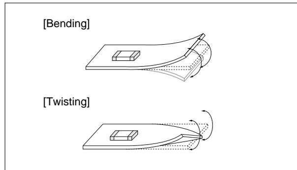
2. Check of the cropping method for the printed circuit board in advance.
