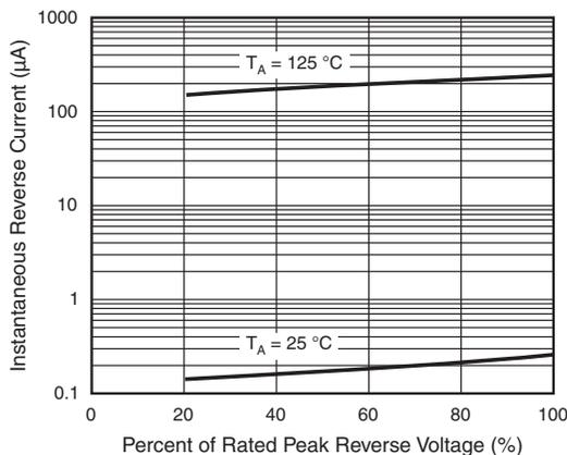
Fig. 4 - Typical Reverse Characteristics Per Diode
