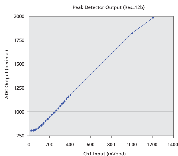
Figure 3-21: Peak Detector Output
