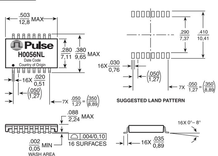
Dimensions:  $\frac{\text{Inches}}{\text{mm}}$  Unless otherwise specified, all tolerances are  $\pm \frac{.010}{0,25}$
