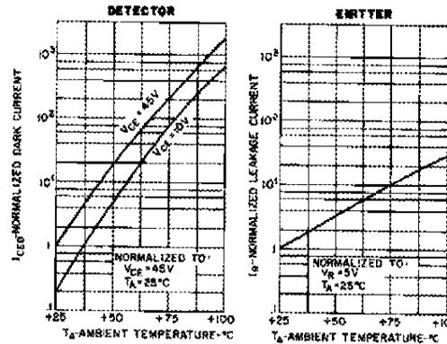
Fig. 4. Leakage Current vs. Temperature ST1145-11
