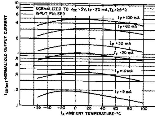
Fig. 2. Output Current vs. Temperature ST1144-11
