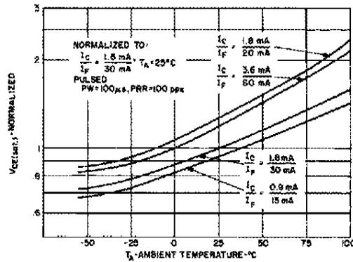
Fig. 3.  $V_{CESAT}$  vs. Temperature ST1141-11
