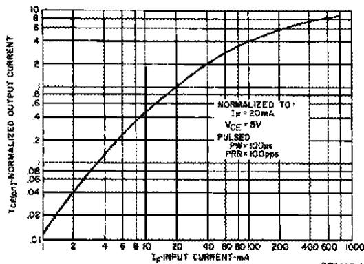
Fig. 1. Output Current vs. Input Current ST1140-11
