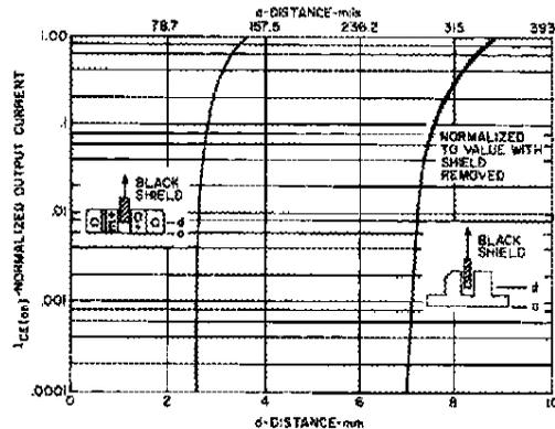
Fig. 6. Output Current vs. Shield Distance ST1143-11
