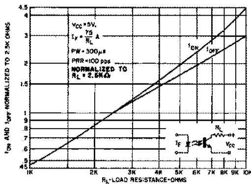
Fig. 5. Switching Speed vs.  $R_L$  ST1142-11
