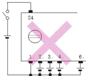
Input Terminals 2, 3, 4, and 6 Connected to the Negative Side of the Power Supply without Being Connected to Power Supply Terminal 1 (\*2)
