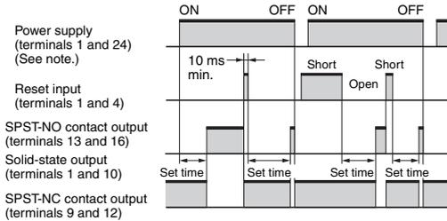
**Note:** When using a 12/24 V DC-operated model with a 12 V DC power supply, short terminals 13 and 15.
