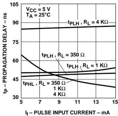
Figure 8. Typical propagation delay vs. pulse input current.
