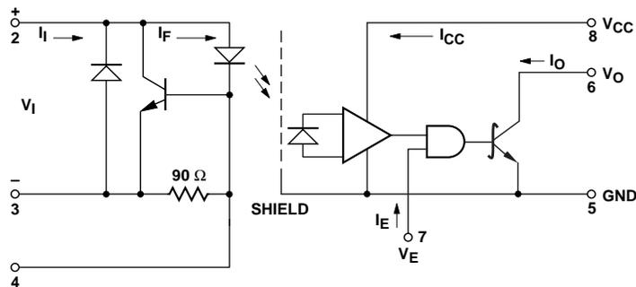
USE OF A 0.1  $\mu$ F BYPASS CAPACITOR CONNECTED BETWEEN PINS 5 AND 8 IS REQUIRED (SEE NOTE 1).
