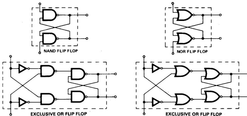
NAND flip flop tolerates simultaneously HIGH inputs; NOR flip flop tolerates simultaneously LOW inputs; EXCLUSIVE-OR flip flop tolerates simultaneously HIGH OR LOW inputs without causing either of the outputs to change.
