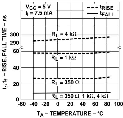
Figure 12. Typical rise and fall time vs. temperature.
