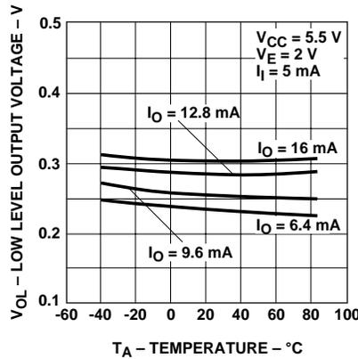
Figure 2. Typical low level output voltage vs. temperature.
