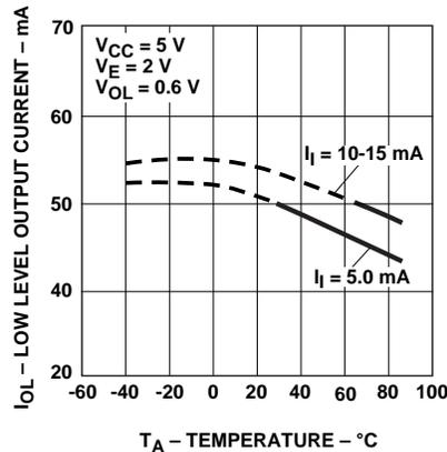
Figure 5. Typical low level output current vs. temperature.
