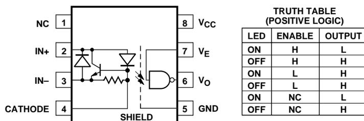
A 0.1 μF bypass capacitor must be connected between pins 5 and 8.
