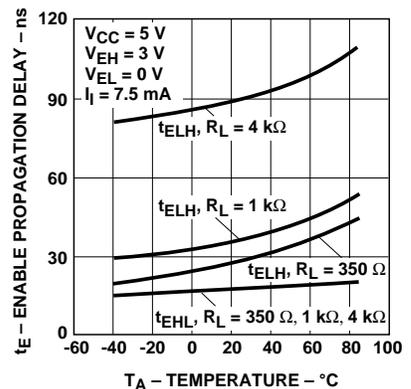
Figure 11. Typical enable propagation delay vs. temperature.
