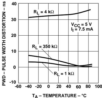
Figure 9. Typical pulse width distortion vs. temperature.
