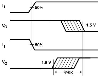
Figure 16. Illustration of propagation delay skew -  $t_{psk}$
