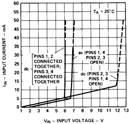
Figure 3. Typical input characteristics,  $I_{IN}$  vs.  $V_{IN}$ .
