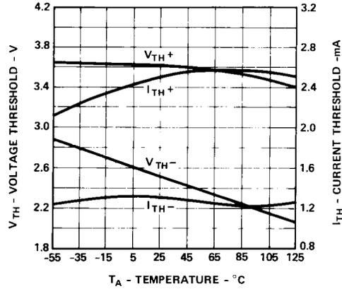
Figure 2. Typical dc threshold levels vs. temperature.
