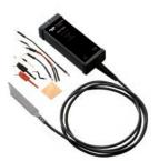
The ZS Series probes provide high impedance and an extensive set of probe tips and ground accessories to handle a wide range of probing scenarios. The high 1  $M\Omega$  input resistance and low 0.9 pF input capacitance mean this probe is ideal for all frequencies. The ZS Series probes provide full system bandwidth for all Teledyne LeCroy oscilloscopes having bandwidths of 1 GHz and lower.
