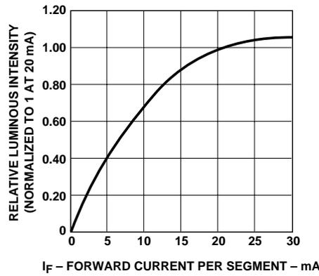
**Figure 2. Relative Luminous Intensity vs. DC Forward Current.**
