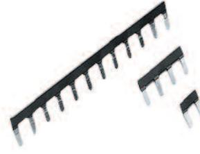
Jumper Pole positions may be removed to provide selective jumpering. When using external jumpers, the terminal's rated cross section is usually reduced one wire size. For jumper maximum current ratings, refer to the corresponding Eurostrip IEC/VDE current rating.
