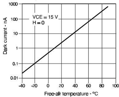
Fig. 6 Collector Current vs Ambient Temperature gra\_076.ds4
